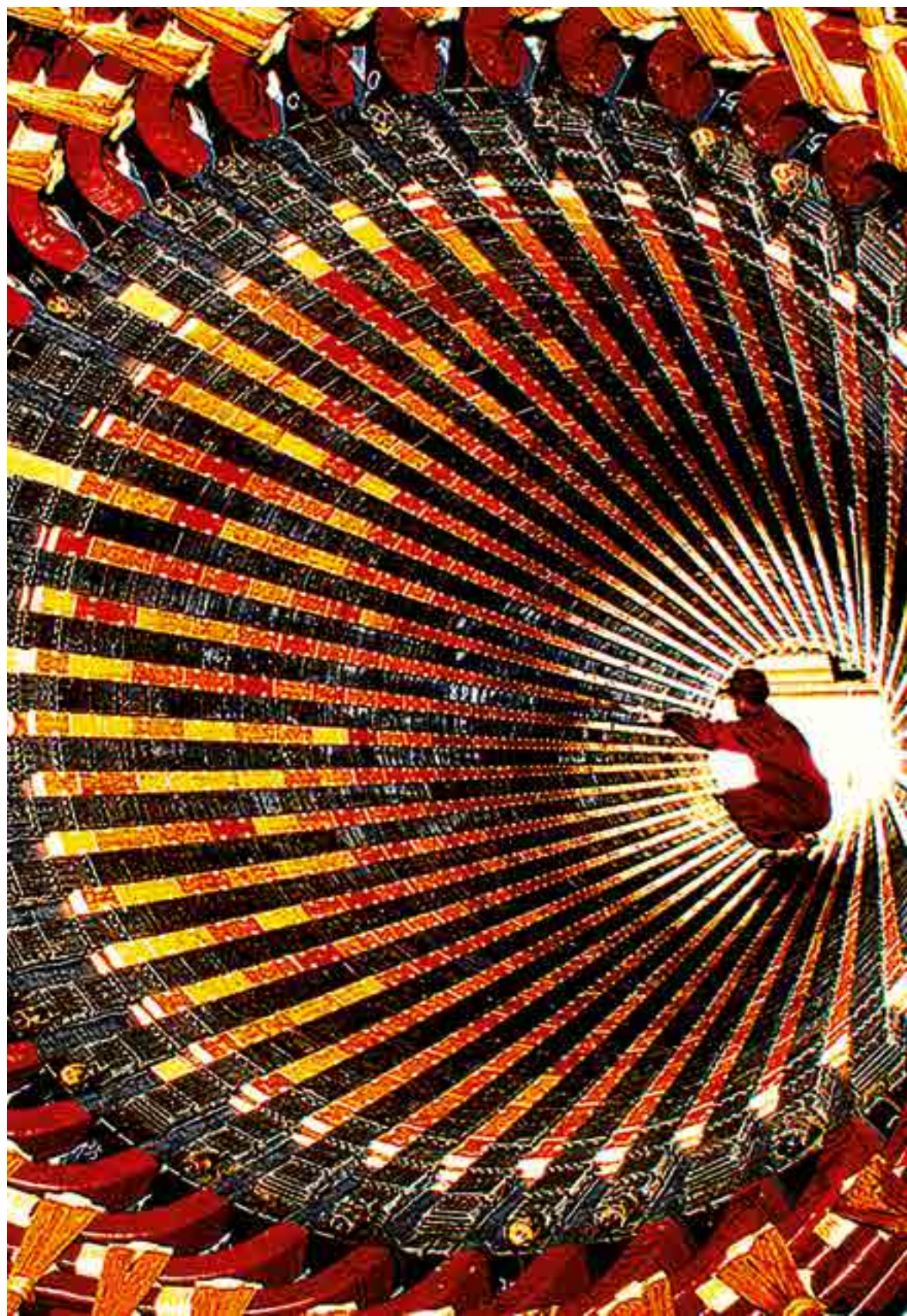
开行融资支持的东方电机大型发电机定子装配现场 CDB-funded Assembling of large generator stator at Dongfang Electric Machinery
